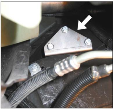
Position the filter mount by placing the tab of the mount into this hole then insert the ground strap bolt and ground strap in the mounting hole of the filter mount and tighten the bolt.
