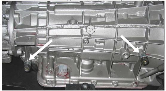
Install by-pass flanges in place of by-pass tube with new Banjo washers. Re-connect the transmission cooler lines to the Banjo Fittings.
