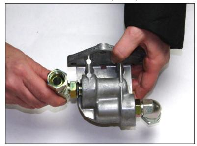
Install the two **90° ORB fittings** into the filter head (<u>do not</u> use pipe sealant). When installed, the fittings need to point in a downwards direction, towards the filter. For ease of installation, we recommend assembling the fittings on the filter head on a work bench before installing it onto the vehicle.
